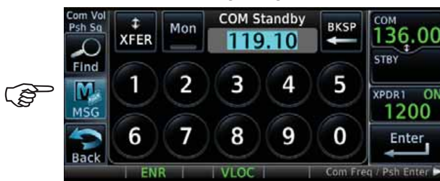
COM Standby Screen
